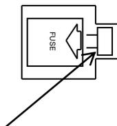
Press this part in the direction of the arrow to take out the fuse. Insert a new fuse until a click sound is heard.
