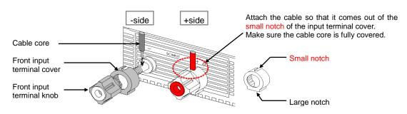
Fig. 4-3 Attaching a Cable without a Crimp Terminal
