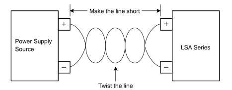
Fig. 4-4 Twisting the Wires of the Load Line
