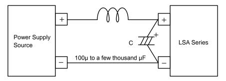
Fig. 4-5 Using a Capacitor to Cancel the Inductance Component
