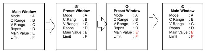
① When you switch from the main window to the preset window, the values displayed in the main window are specified as the values for the unit.
