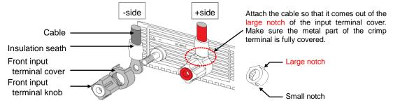
Fig. 4-2 Attaching a Cable with a Crimp Terminal
