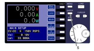
3 Press the "Mode" DIRECT key in the MAIN SETUP window. At this time, the ENTER key begins to flash green.
