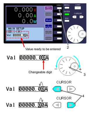
Press the DIRECT key next to the "Main Setup" icon to display the MAIN SETUP window.
