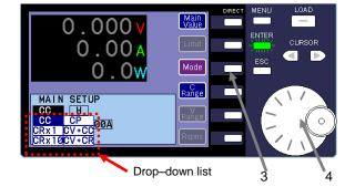
3 Press the "Mode" DIRECT key in the MAIN SETUP window. At this time, the ENTER key begins to flash green.
