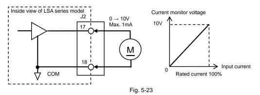
\* When you switch the unit on and off, the current monitor circuit becomes unstable. As a result, voltage might be generated by current monitor output.
