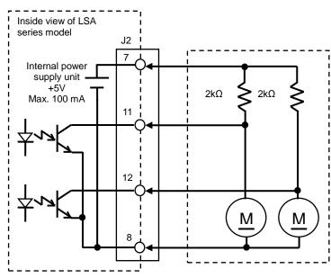
You can use the J2 connector pin No. 7 and an external resistance to output the C Range status of the unit as voltage. The values for the figure on the left are as follows:
