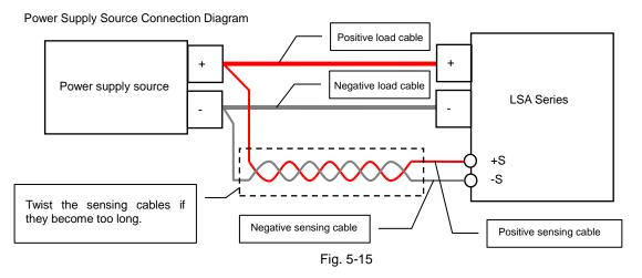
Very little current is actually applied to the voltage remote sensing cables. However, it is important to use cables capable of withstanding the voltage that is output by the power supply voltage. We recommend using cables with twisted AWG24-28 wires.
