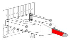
There is only one rear input terminal cover for the LSA-165 and LSA-330.
