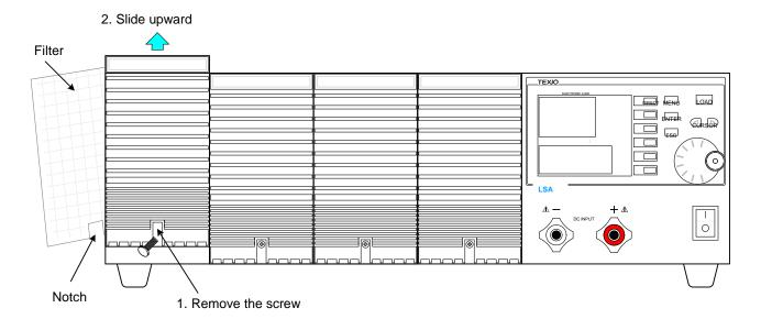
Fig. 4-6 Removing the Front Grill
