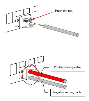
Push and hold the  $\pm$ S connector tab, then insert the cable into the hole to the left of the tab.
